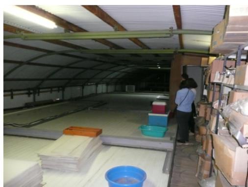
**Figure 2** Combustible materials stored adjacent to the cold storage unit
